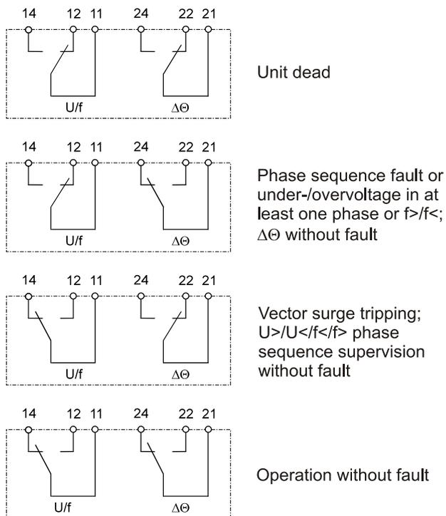
Figure 2.2: Contact positions of the output relays
