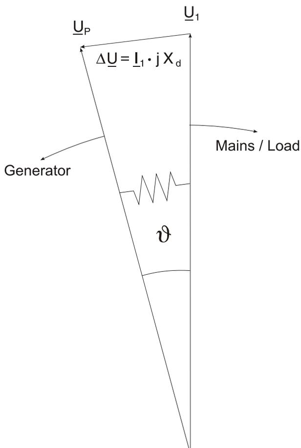
Figure 3.2: Voltage vectors at mains parallel operation
